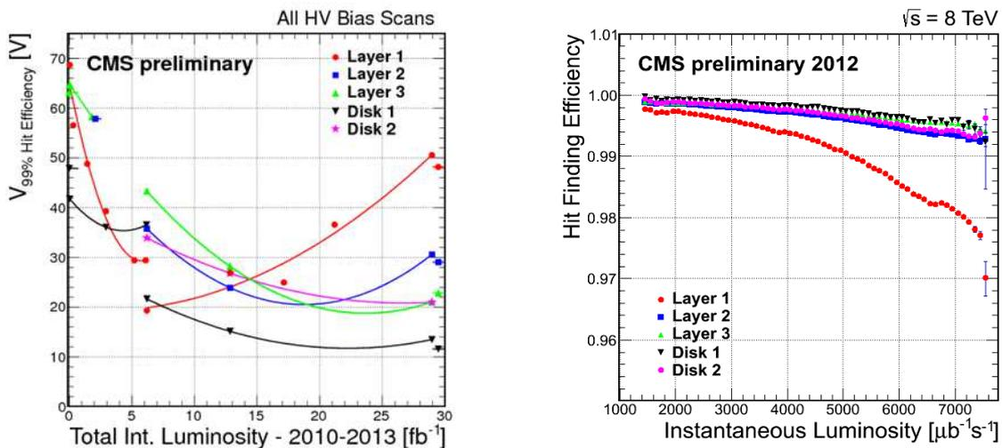
**Figure 2:** Pixel measurement efficiency in various tracking layers of the detector — **Left:** as a function of total integrated collision data, and **Right:** as a function of instantaneous luminosity
