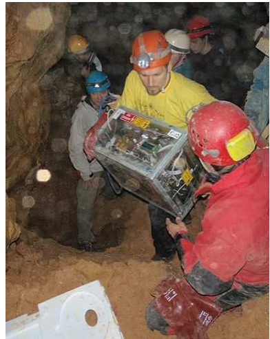
Fig. 6: The portable Muon Tomograph in the Ajándék-cave
